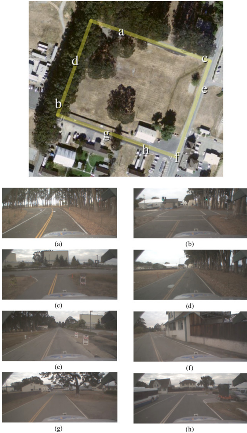
Fig. 16 Aerial view of test track. The transparent yellow line represents the 560-meter square loop in which we tested our vehicle. The letters indicate correspondence with the lower figures as seen from the vehicle. Note that GPS coverage is minimal along the east and north segments of the loop with areas where no satellites are observed.
