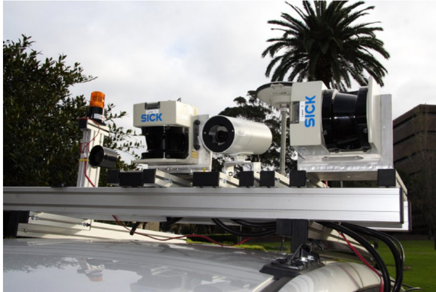
Fig. 6 The sensor suite: SICK lasers, INS, and camera.
